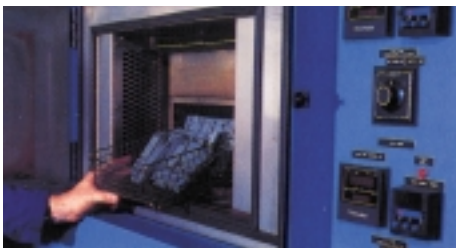
IGNITION COMPONENTS ARE TESTED FOR FUNCTIONAL STABILITY UNDER EXTREME VARIATIONS IN WELLS' TEST LABS.
